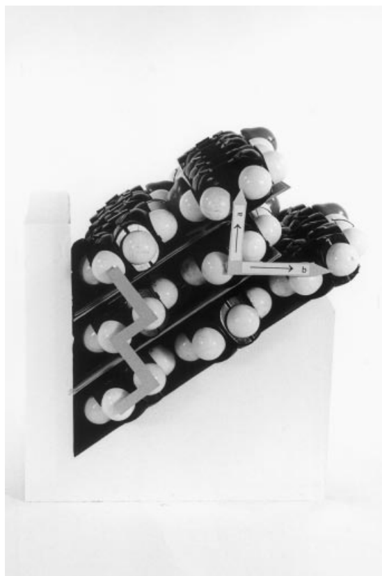
Fig. 10. Clinographic edge-on-view perpendicular to the F-face of beta-quinacridone. The two stairs (left, grey) indicate the \pi – \sigma correlation of three adjacent molecules. a - and b -axes are marked. The photo shows the end-over position of quinacridone molecules represented by real space-filling models.
