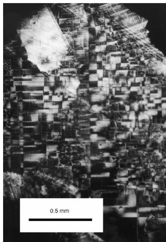
Fig. 7. Crystal of beta-quinacridone grown in boiling xylene, observed under polarized light.
